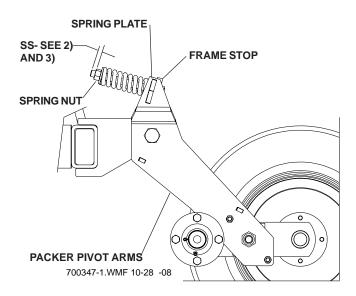
1) WITH THE MAIN FRAME LEVEL TIGHTEN THE SPRING BOLT TO A (SS) DISTANCE OF APPROXIMATELY 3/8"-1/2" ON ALL THE MAIN FRAME PACKERS.
