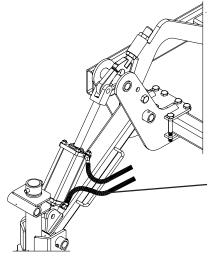
NOTE: CYLINDERS ON FRONT LIFT AXLES MUST BE MOUNTED WITH RODS UP AND PORTS TO THE SIDE. CYLINDERS ON THE REAR PACKER LIFT SHOULD BE MOUNTED WITH THE RODS UP. REMOVE AND ROTATE END GLANDS IF REQUIRED. FAILURE TO ORIENTATE AS INDICATED CAN CAUSE PORT INTERFERENCE, CHECK FOR INTERFERENCE, BEFORE AND WHILE ACTIVATING ALL CYLINDERS.
