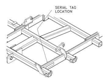
When in need of parts, always specify the model and serial number. Write this number in the space provided.
