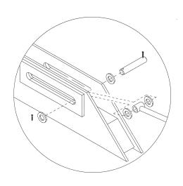
NOTE: A 2 ½ FOOT LONG EXTENSION BOLTS BETWEEN THE CYLINDER AND THE MOUNT ON THE MAIN FRAME. ATTACH WITH U-BOLTS.
