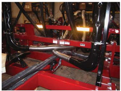
Mount two monitor modules to the main frame of the drill. The modules are labeled "Art module" and "three load module." Use self-tapping screws and mount on the left side of the center front-to-rear member on the main frame. Mount on module plate mounted to rear hitch mounting bolts. The modules plug into each other.
