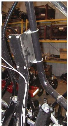
Manifold offset bracket. Used on inside manifold on each wing.
