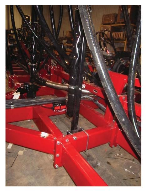
Offset manifolds about 2-inches in height to make it easier to install the 4-inch flexible hoses.
