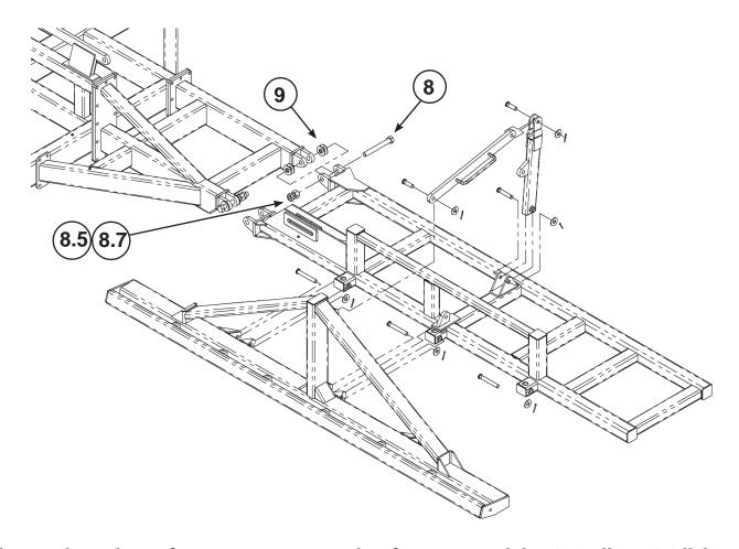
Attach wing frames to main frame with 1 ¼" x 10" bolts (Item 8). Each bolt is secured with a regular nut and a narrower jam nut (Items 8.5 and 8.7). Bolts should only be snugged up until there is no side to side play. Do not tighten against ears. Tighten jam nut securely against regular nut.
