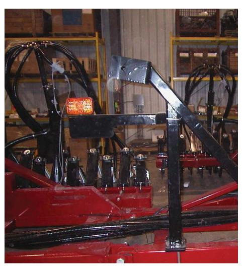
vehicle mount bracket that hangs under the rear hitch. See photos for placement details.
