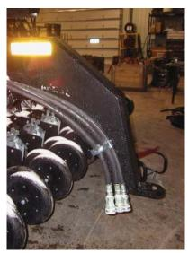
Two flat brackets attach to the bottom of the rear hitch to support hoses. Attach to hitch with u-bolt and attach hoses to bracket with clamp and 3/8" bolts. Attach hoses to rear hitch with hydraulic hold down clamp and 3/8" bolt.
