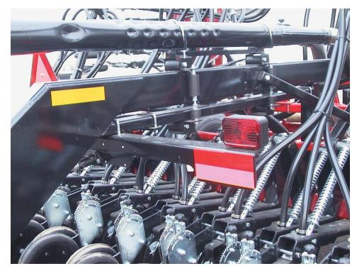
Bracket attaches with u-bolt to rear hitch.
