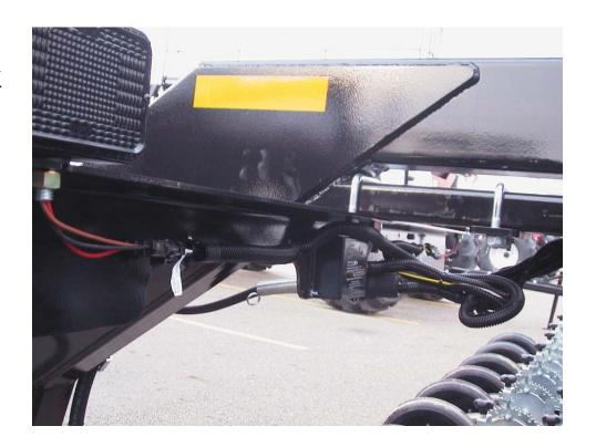
Mount the remote work switch on drill - it mounts to a bracket near the left main frame tire. (Item A on diagram below) Connect a 4 meter minidin cable (small black monitor wire) to the work switch and plug it into any port on the bottom of the 3-load or flow module in the center of the drill. There are two locations on each module to plug in sensors (it doesn't matter which one you use).
