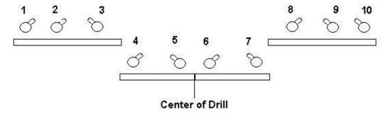
Manifold 1 - Mount between row units 5 and 6 from left end of drill. Point outlet as shown
