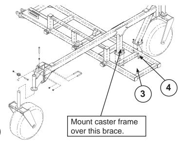
is mounted over the front rank of the wing frame. The rear (straight) leg is mounted over the 4 x 4 front to rear frame brace member. This is the third front to rear brace from the end.
