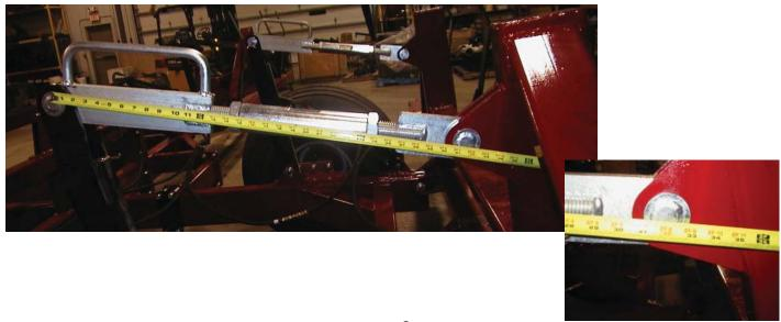
Attach caster frames to wing frames using ¾" u-bolts (Item 3) and lock nuts (Item 4).
