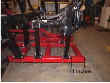
Mount straight stand just inside front to rear frame member. Attach with 5/8" u-bolts but do not tighten.
