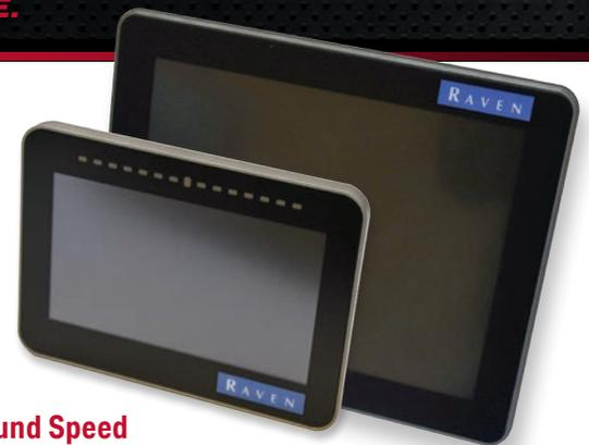
**Monitor Functions:** > Fan Speed > Bin Levels > Meter Status > Blockage > Ground Speed
